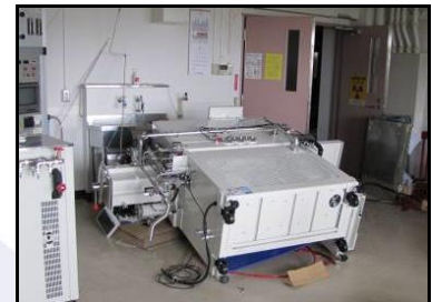
Equipment impacts: toppled unrestrained lab workstations
